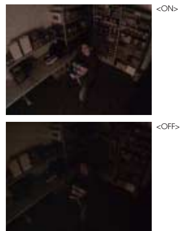
Fig. 3 (actual images) Light Funnel Function in 0.3 lx lighting conditions * When the light funnel function is activated, the image resolution is 640 x 480 (VGA).
